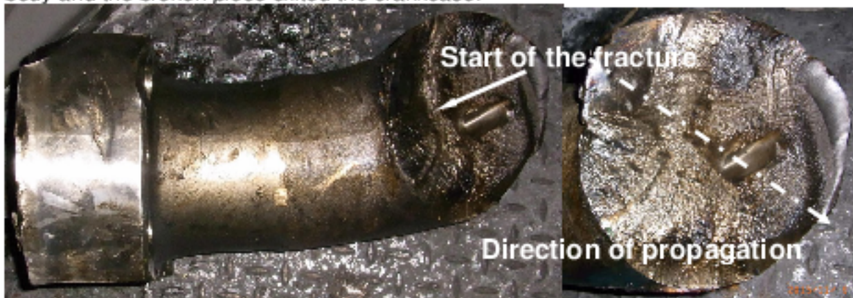
Figure 14: Broken connecting rod with detailed enlargement of the broken surface
