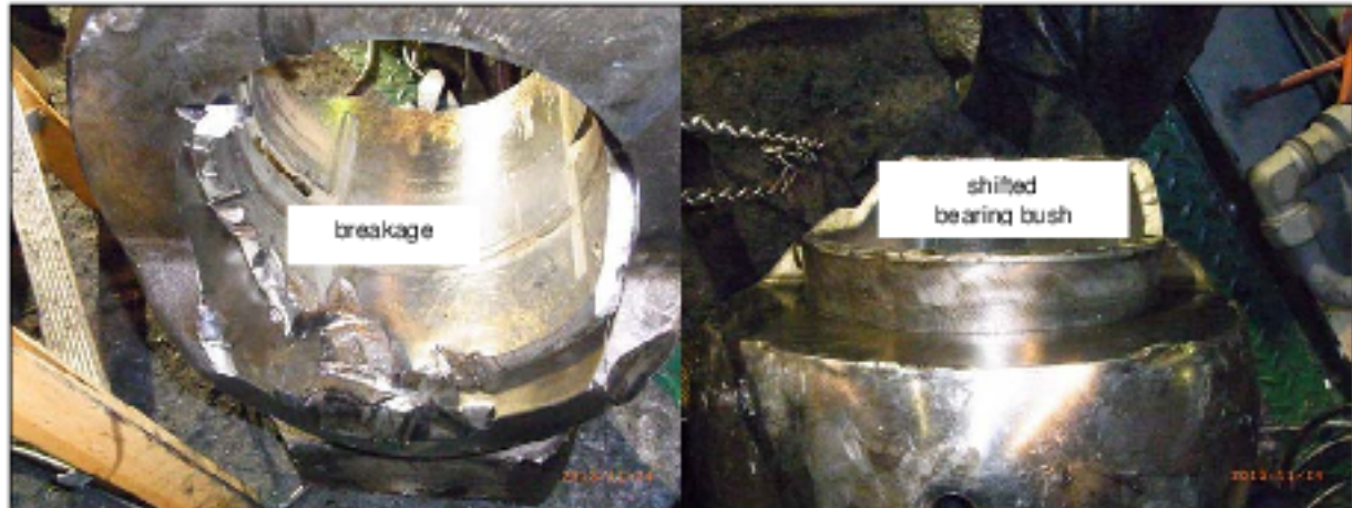
Figure 13: Connecting rod eye with breakage and laterally shifted bearing bush
