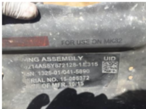
Figure C.60.5 Component from a Paveway laser guidance system wing
