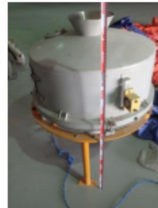
Figure D.36.8 Heating vessel
