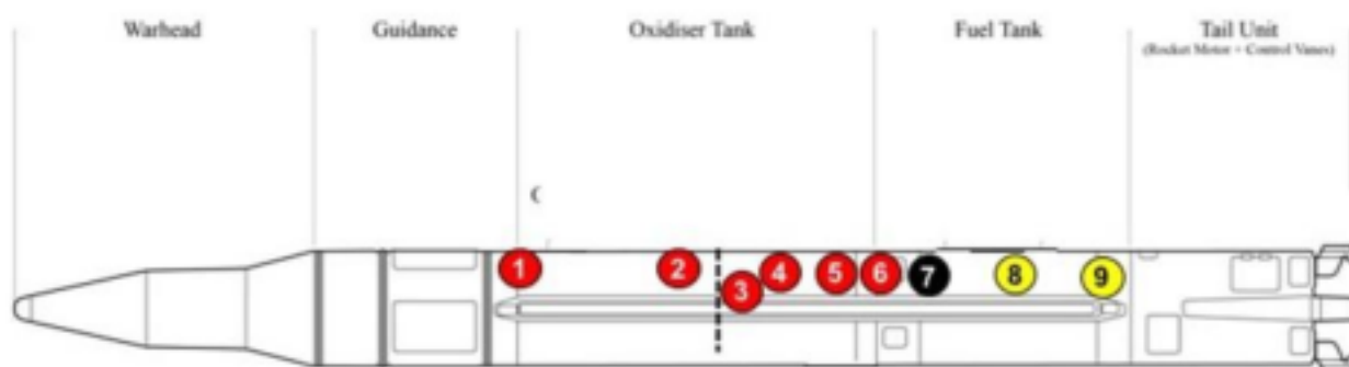
Figure VI Illustrative main section layout of an extended-range short-range ballistic missile a
