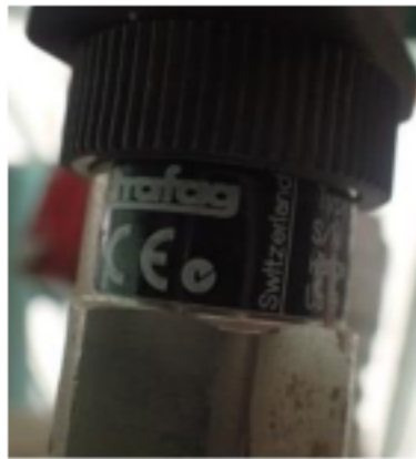
Figure D.36.23 E C T 8472 Industrial Pressure Transmitter (Traced: Member State > IR)
